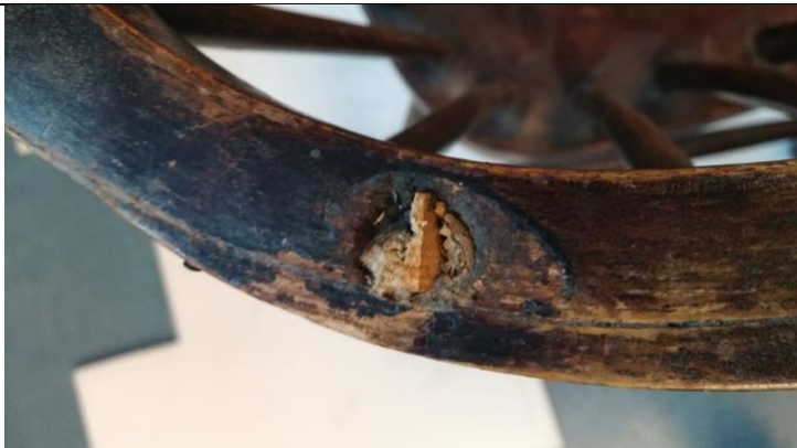
e. Dirty, stained surface, broken off dowels/biscuit join on right arm rail
