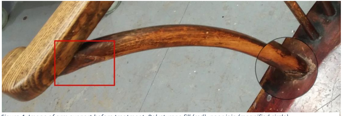
Figure 4. Image of arm support before treatment. Polystyrene fill (red), poor join (magnified circle).
