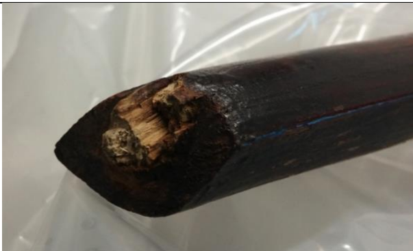
c. Top rail (right), broken half of dowel still embedded
