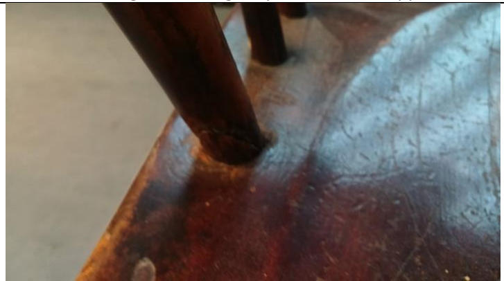
f. Wedge repair (right arm support)
