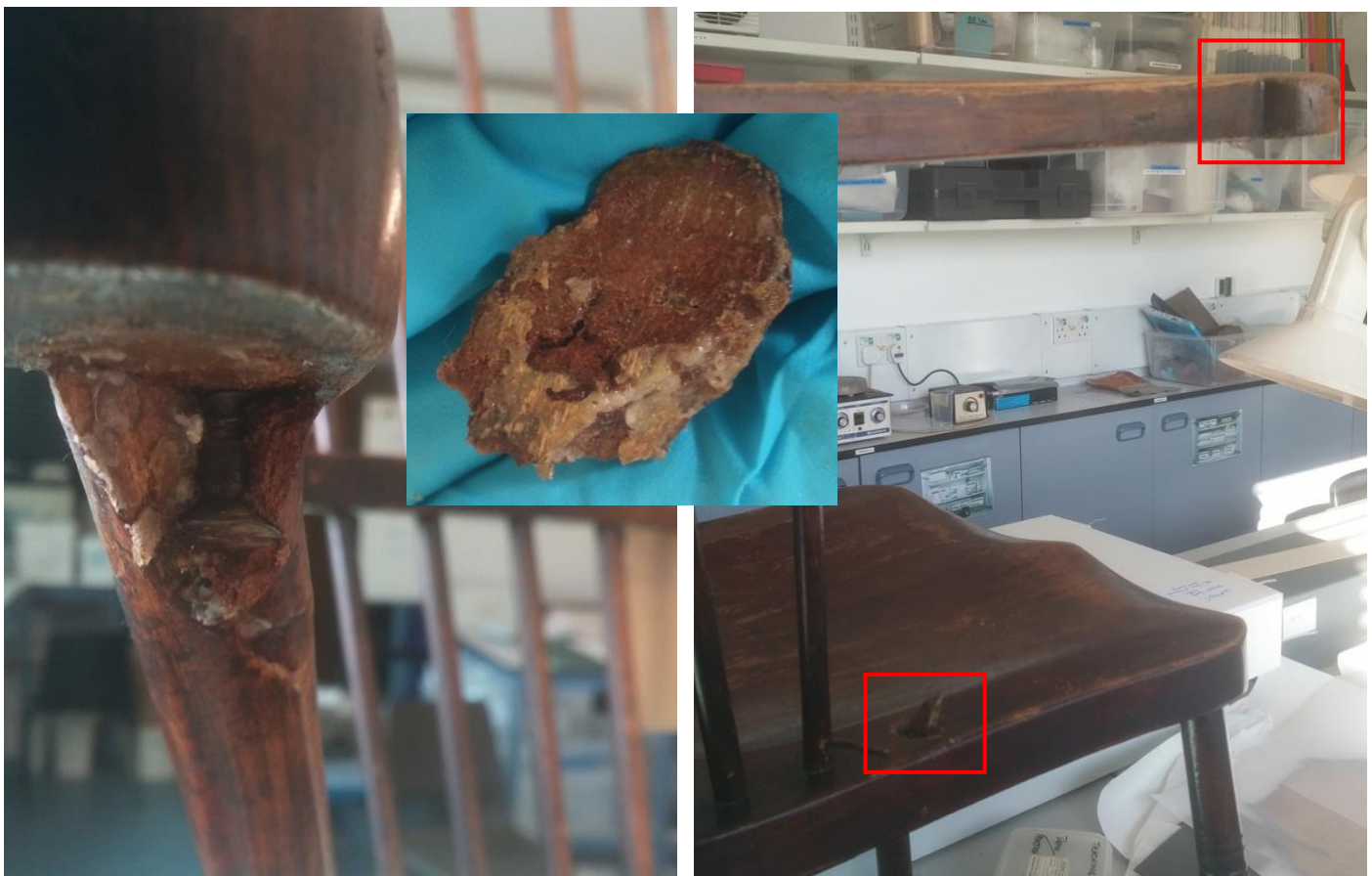
Figure 5. Polystyrene fill (left, middle). Chair after right arm support was removed (right).
